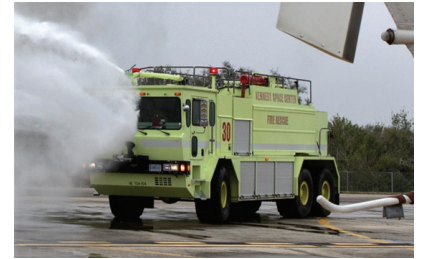
All air rescue fire fighting trucks at KSC were retrofitted and equipped to collect and recycle AFFF.
